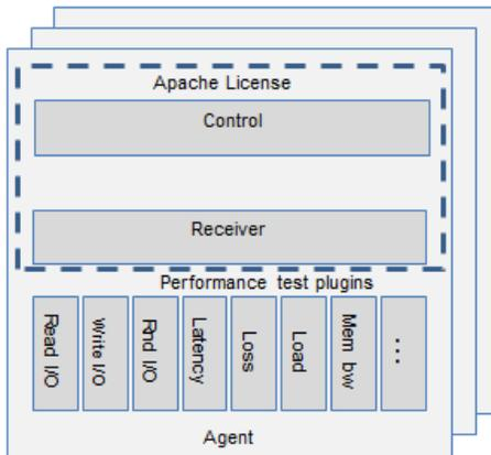
The agent VM is installed in the cloud platform to perform its platform monitoring task. Each agent holds a number of test plug-ins. Each test plug in performs a specific test (IO read / write, Storage, Web look up, TWAMP etc).
